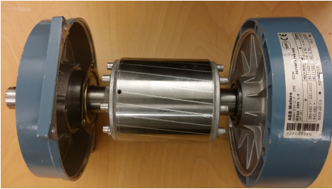
Figure 7. Detail of the motor used in our experiments: the broken rotor bar fault has been artificially produced by drilling a hole in the squirrel cage.
